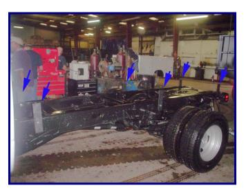
2. Install the straps using the supplied <sup>1</sup>/<sub>2</sub>' x 1 <sup>1</sup>/<sub>2</sub>" bolts, flat washers, lock washers and nuts. You will find it helpful to install the bolts so the nuts are to the outside of the truck frame. This will make it easy to tighten the nuts and will also make final inspection possible from the outside of the truck frame. Snug bolts just enough to keep the mounting straps standing straight up. Watch for wires, hoses or brake lines inside the frame.
