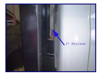
Weld each body mounting strap to the channel long sills on all three sides.
